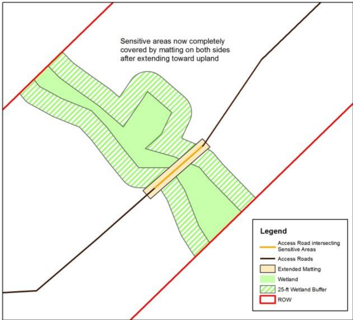
Figure 15. Extension of Access Road Matting Example – Part 2
