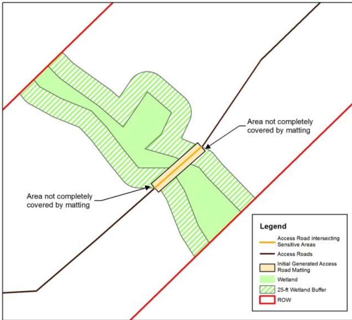
Figure 14. Extension of Access Road Matting Example - Part 1
