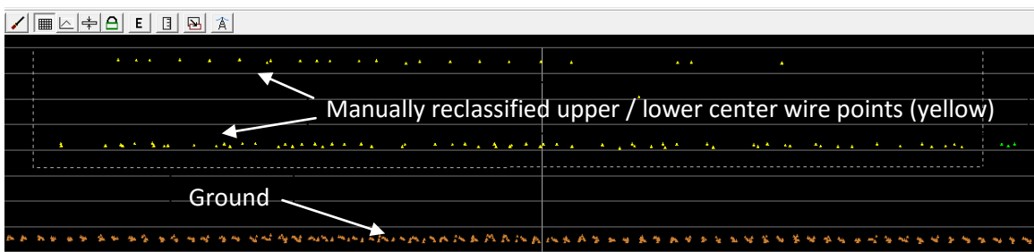
Figure 3.29 – Manually reclassified upper / lower center wire points (yellow)
