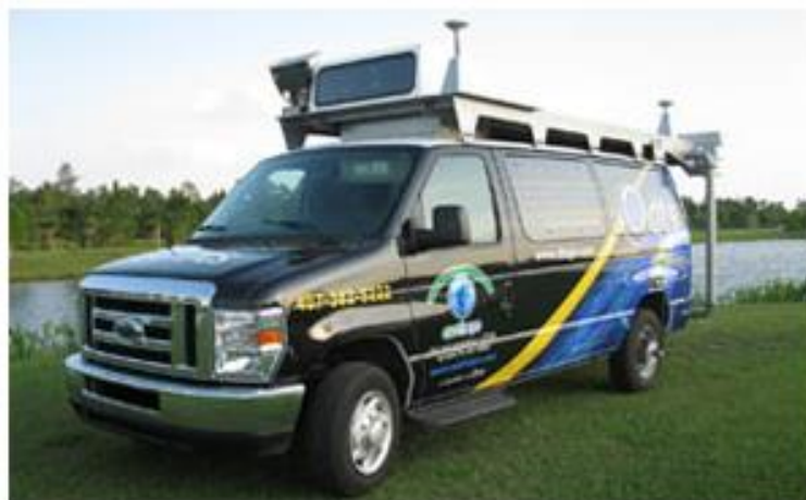
Figure 2.2 – Example of a mobile LiDAR sensor mounted atop a van (Photo by Earth Eye, LLC)
