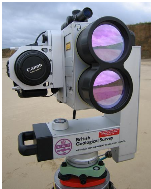
Figure 2.4 – A stationary terrestrial LiDAR system (British Geological Survey. Non-commercial use license - https://www.bgs.ac.uk/about/copyright/non-commercial_use.html )
